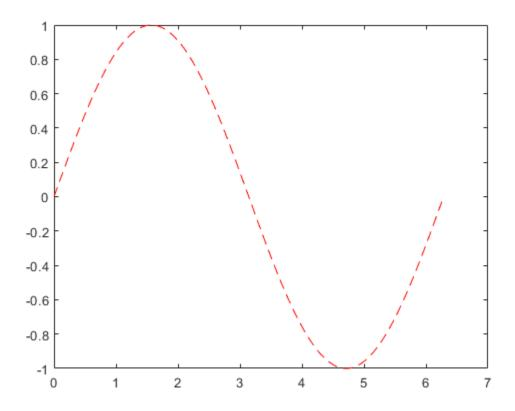
'r--' is a *line specification*. Each specification can include characters for the line color, style, and marker. A marker is a symbol that appears at each plotted data point, such as a +, 0, or \*. For example, 'g:\*' requests a dotted green line with \* markers.
